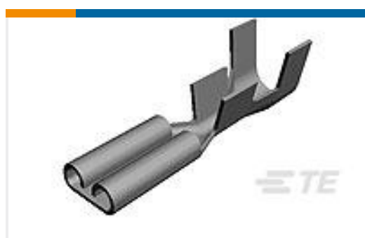
TE Part #41772-1 250 FASTON REC 22-18 AWG BR
