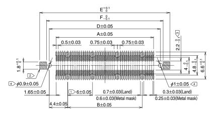
Note 1 Cross-hatched portions, totaling n places, indicate the ground circuits.
