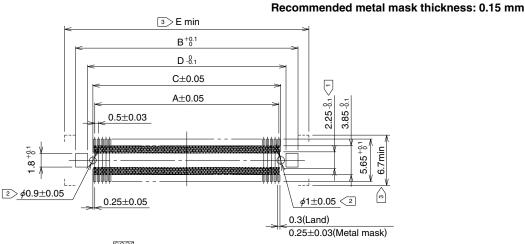
Note The cross-hatched area inside the SMT land may come into contact with the connector contacts and thus care should be taken that the pattern does not extend beyond the SMT land width.
