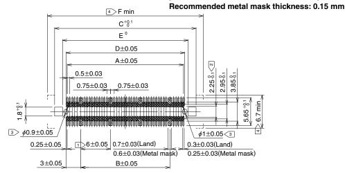
Note 1 Cross-hatched portions, totaling n places, indicate the ground circuits.
