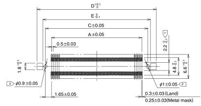
Note 1 The cross-hatched area inside the SMT land may come into contact with the connector contacts and thus care should be taken that the pattern does not extend beyond the SMT land width.
