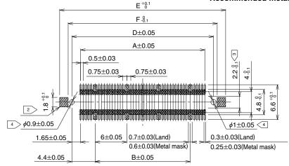
Note 1>Cross-hatched portions, totaling n places, indicate the ground circuits.
