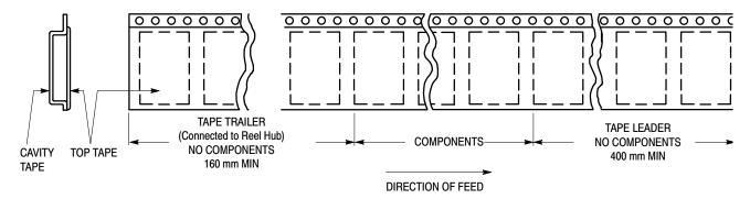
Figure 10. Tape Ends for Finished Goods
