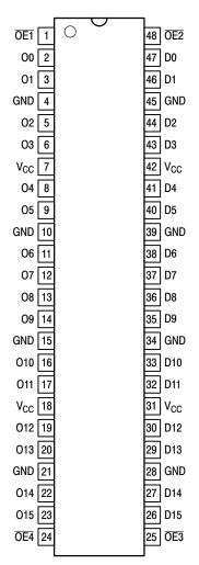
Figure 1. 48-Lead Pinout (Top View)
