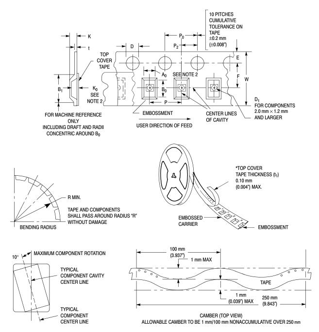
Figure 7. Carrier Tape Specifications
