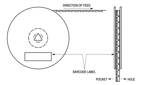
Figure 9. Reel Winding Direction
