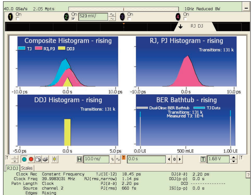
Figure 1: Jitter Analysis of a QT84LD-40MHZ
