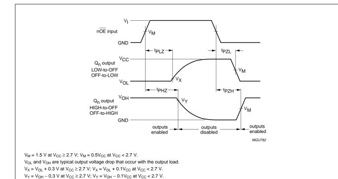
Fig.6 3-state enable and disable times.
