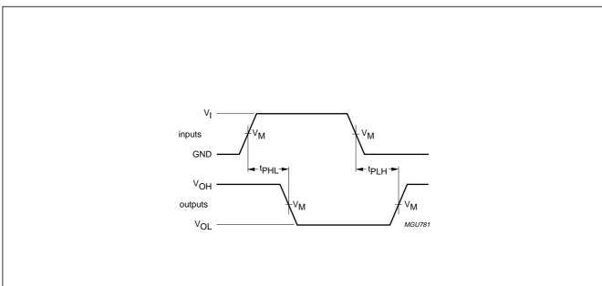
$V_M$  = 1.5 V at  $V_{CC} \geq$  2.7 V;  $V_M$  = 0.5V  $_{CC}$  at  $V_{CC}$  < 2.7 V.
