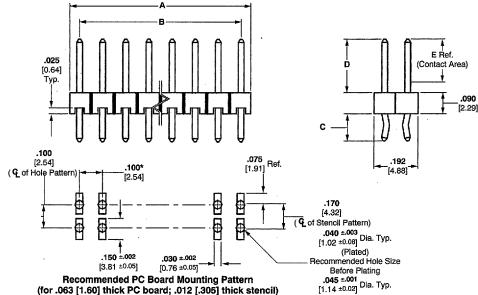
Recommended PC Board Mounting Pattern (for .063 [1.60] thick PC board; .012 [.305] thick stencil) \*±.003 [±0.08] tolerances not to accumulate within one connector pattern.
