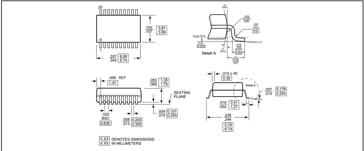
20-Pin 300 Mil-Wide Plastic SOIC (S) Package
