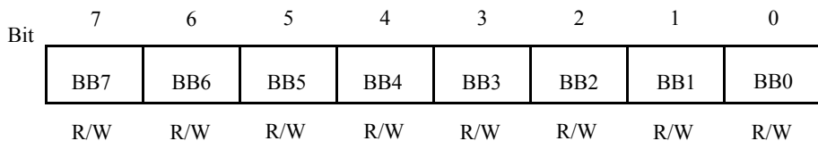
Figure 74. MMU Bank Base Register (BBR: I/O Address = 39h)
