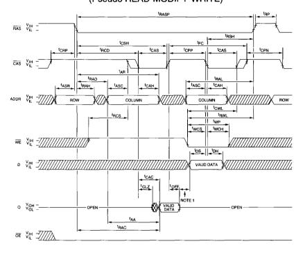
NOTE: 1. Do not drive data prior to High-Z; that is completion of ¹OFF. ¹CPP is equal to ¹OFF + ¹DS(MIN) + guardband between data-out and driving new data-in.
