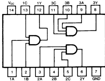
Suffix-Blank: Plastic Dual In Line Package
