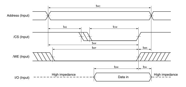
Cautions 1. /CS or /WE should be fixed to high level during address transition.
