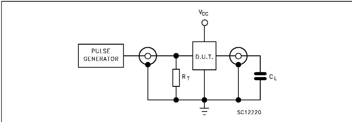
$C_L = 15/50 \text{ pF}$  for equivalent (includes jig and probe capacitance)
