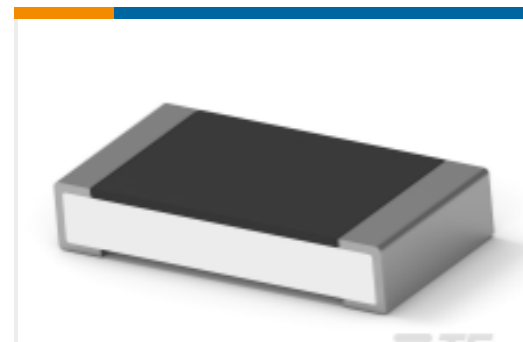
TE Part #4-2176391-7 RQ 1206 37K4 0.1% 10PPM 5K RL
