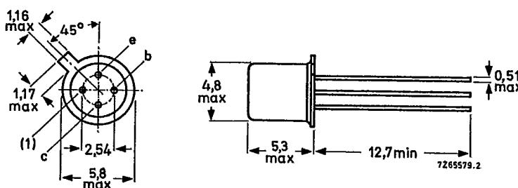
(1) = shield lead (connected to case).
