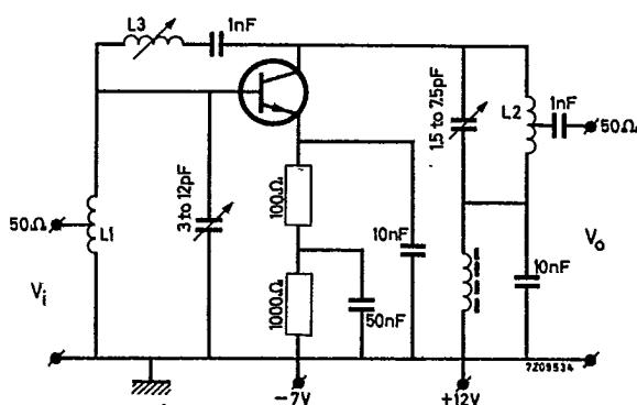
$L_1 = 3,6$  turns tinned Cu wire, 1,3 mm
