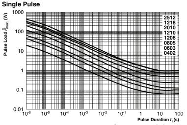
Maximum pulse load, single pulse; applicable if  $\overline{P} \rightarrow 0$  and n < 1000 and  $\hat{U} \le \hat{U}_{max}$ ; for permissible resistance change equivalent to 8000 h operation
