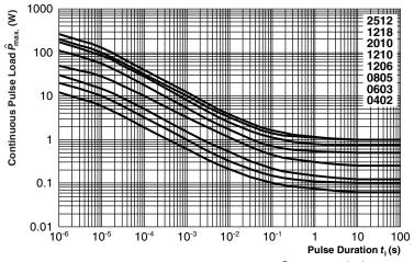
Maximum pulse load, continuous pulses; applicable if  $\overline{P} \le P(9_{amb})$  and  $\hat{U} \le \hat{U}_{max}$ ; for permissible resistance change equivalent to 8000 h operation
