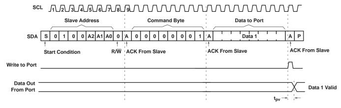
Figure 6. Write to Output Port Register
