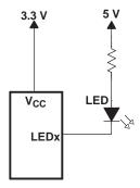
Figure 16. Device Supplied by a Lower Voltage
