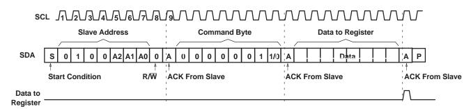
Figure 7. Write to Configuration or Polarity Inversion Registers
