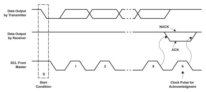
Figure 3. Acknowledgment on I<sup>2</sup>C Bus
