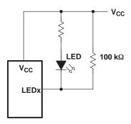
Figure 15. High-Value Resistor in Parallel With the LED
