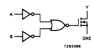
Fig.5 Logic diagram (one gate).
