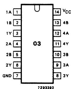
Fig.1 Pin configuration.
