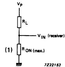
(1)  $R_{ON(max)} = 0.26 \text{ V} / 4 \text{ mA} = 65 \Omega$  (at 25 °C)
