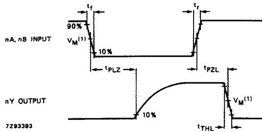
HC:  $V_M = 50\%$ ;  $V_I = \text{GND to } V_{CC}$
