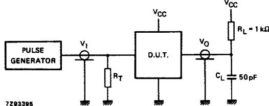
Fig.7 Test circuit (open drain)
