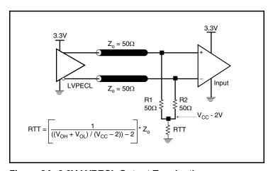
Figure 3A. 3.3V LVPECL Output Termination
