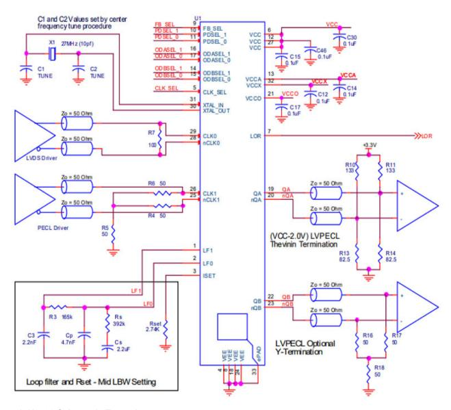
Figure 5. 813N2532 Schematic Example
