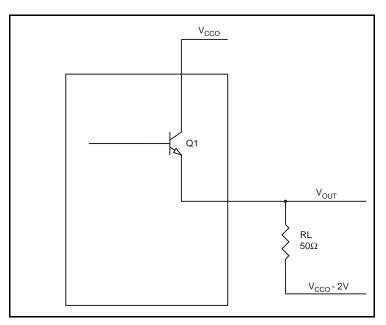
Figure 6. LVPECL Driver Circuit and Termination
