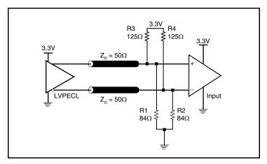
Figure 3B. 3.3V LVPECL Output Termination
