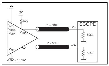
3.3V LVPECL Output Load AC Test Circuit
