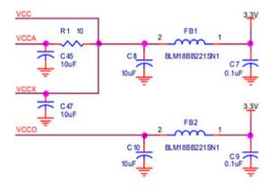
Place each 0.1uF bypass cap directly adjacent to its corresponding VCC, VCCA, VVCCX or VCCO pin.
