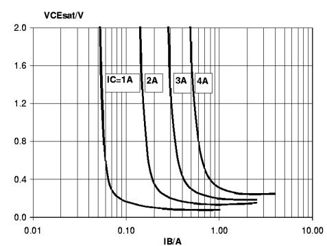
Fig.10. Collector-Emitter saturation voltage.
