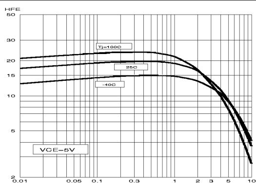
Fig.9. Typical DC current gain.  $h_{FE} = f(I_C)$
