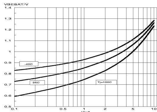
Fig.11. Base-Emitter saturation voltage.
