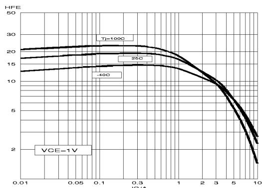
Fig.8. Typical DC current gain.  $h_{FE} = f(I_C)$
