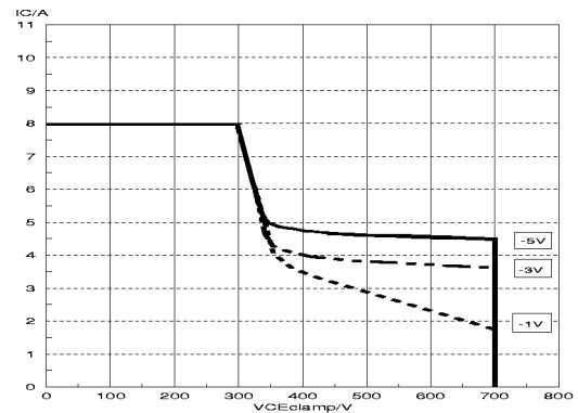
Fig.15. Reverse bias safe operating area ( $T_j < T_{jmax}$ )
