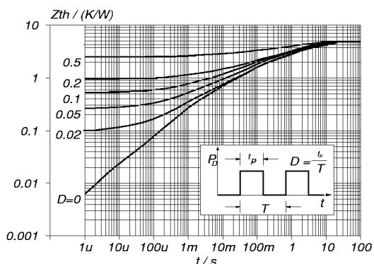
Fig.13. Transient thermal impedance.
