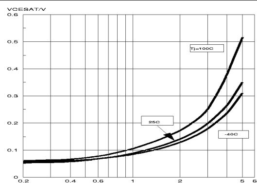
Fig.12. Collector-Emitter saturation voltage.
