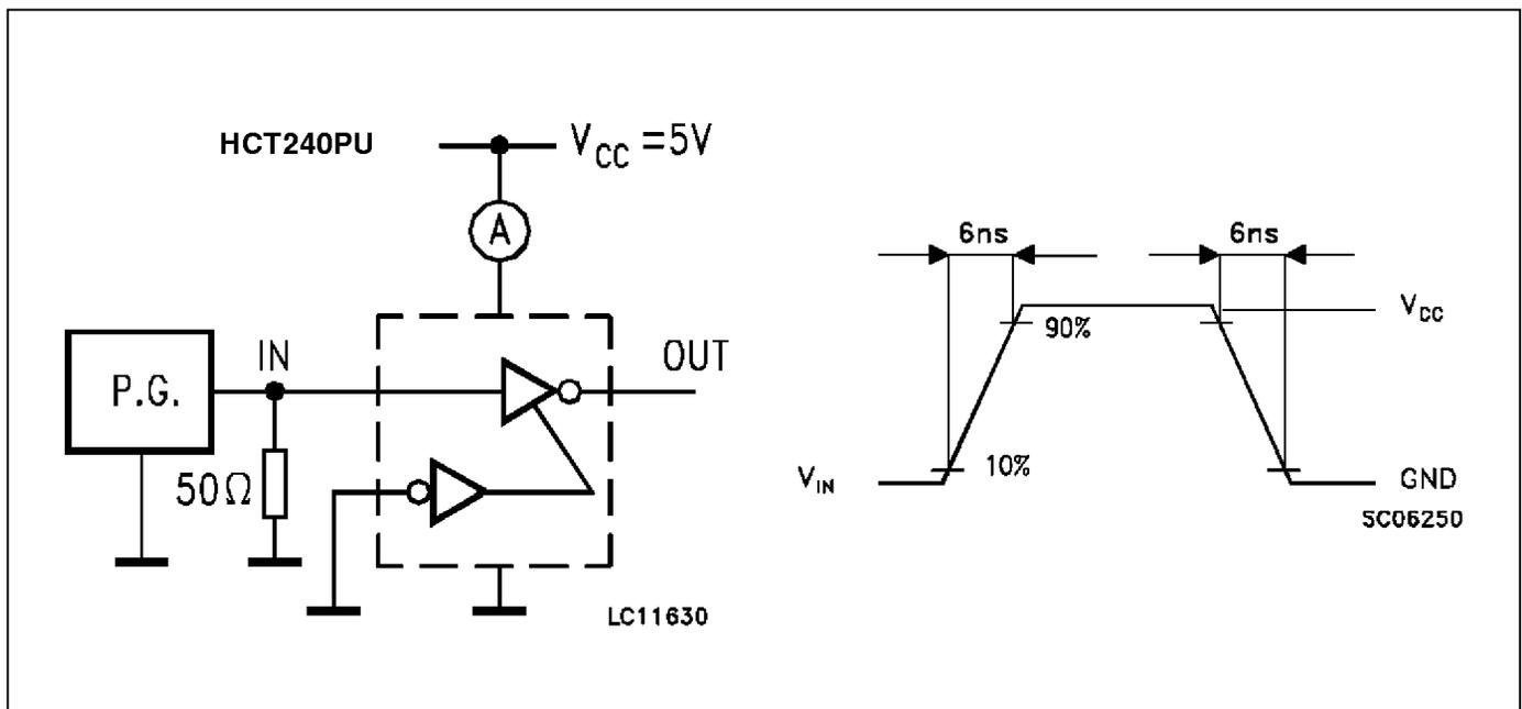
SWITCHING CHARACTERISTICS TEST WAVEFORM
