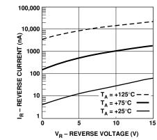
Figure 2. Reverse Current vs. Reverse Voltage at Temperatures.
