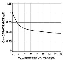
Figure 4. Total Capacitance vs. Reverse Voltage.
