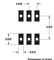
Figure 7. Recommended PCB Pad Layout for Avago's SC70 6L/SOT-363 Products.
