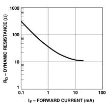
Figure 3. Dynamic Resistance vs. Forward Current.
