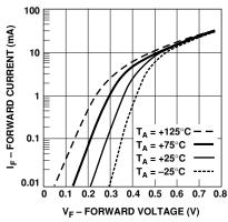
Figure 1. Forward Current vs. Forward Voltage at Temperatures.
