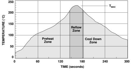
Figure 8. Surface Mount Assembly Profile.
