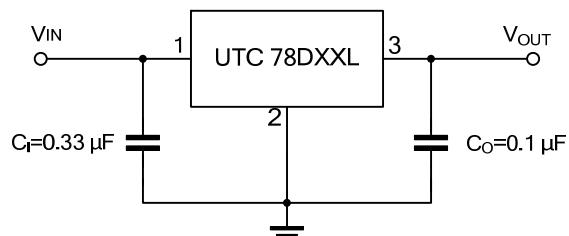
Note: Bypass capacitors are recommended for optimum stability and transient response and should be located as close as possible to the regulators.
