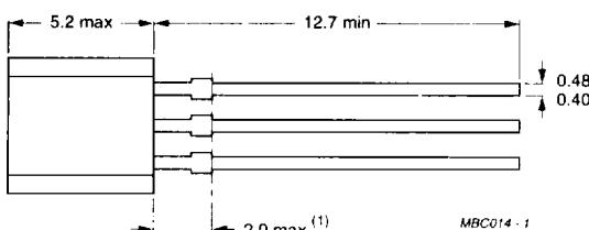
Note (1) Terminal dimensions within this zone are uncontrolled to allow for plastic and terminal irregularities.
