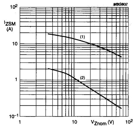
Fig.3 Non-repetitive peak reverse current as a function of the nominal working voltage.
