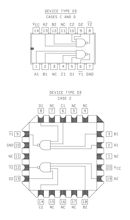
FIGURE 1. <u>Terminal connections and logic diagram</u> Continued.
