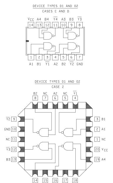
FIGURE 1. Terminal connections and logic diagram (top view).
