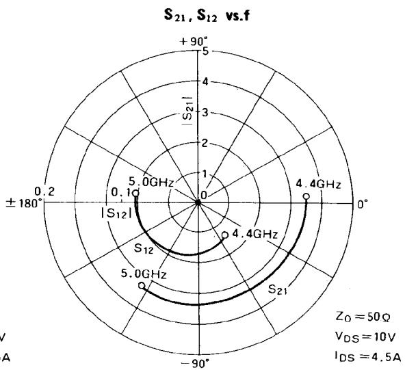
**S PARAMETERS ( $T_a = 25^\circ\text{C}$ ,  $V_{DS} = 10\text{V}$ ,  $I_{DS} = 4.5\text{A}$ )**
