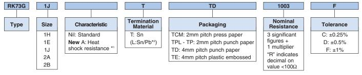
\*1 With type A, only T is available as the terminal surface material.
