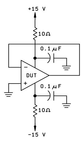
FIGURE 2. Radiation exposure circuit.
