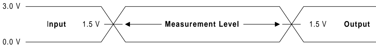
Figure 14. Input Waveforms and Measurement Levels
