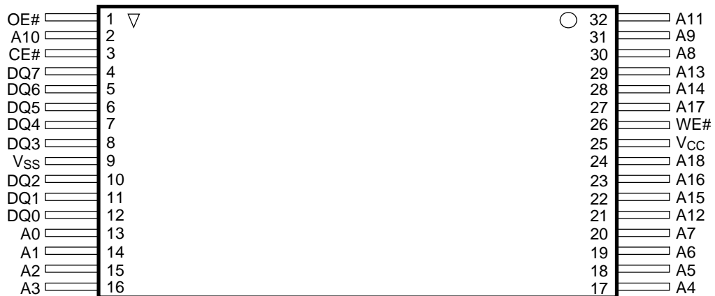
32-Pin Reverse TSOP
