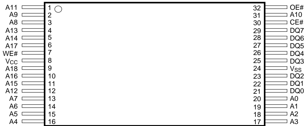
32-pin Standard TSOP
