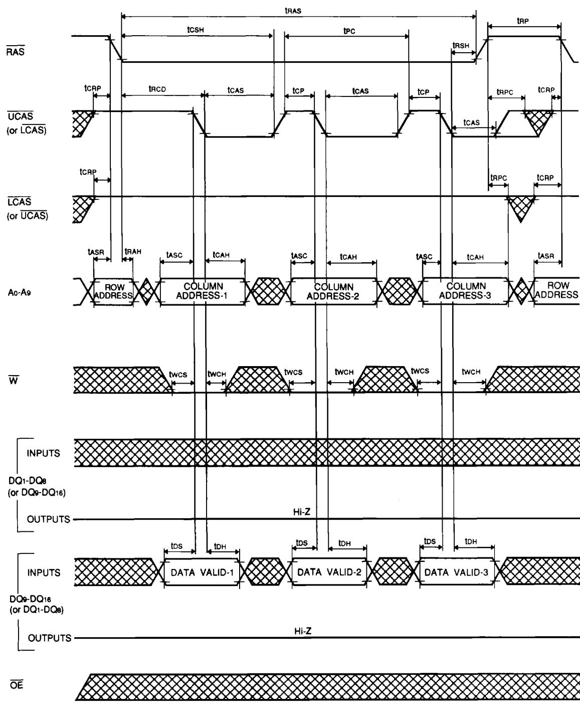
Fast Page Mode Write Cycle ( Delayed Write )
