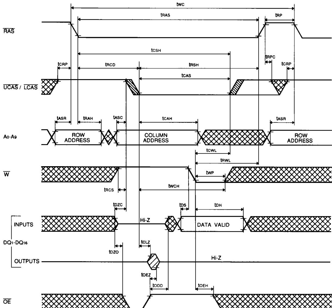
Upper/(Lower) Byte Write Cycle ( Delayed write )
