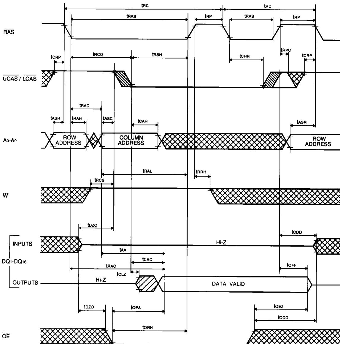
Note 29: Early write, delayed write, read write or read modify write cycle is applicable as well as read cycle.
