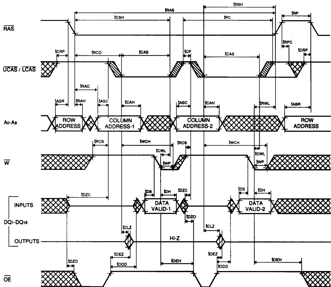
Fast Page Mode Upper / (Lower) Byte Write ( Delayed Write )
