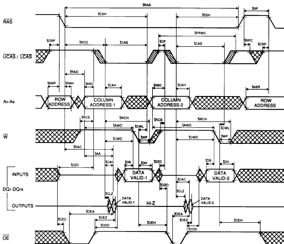
Fast Page Mode Read-Upper/(Lower) Write, Read-Modify-Upper/(Lower) Write Cycle
