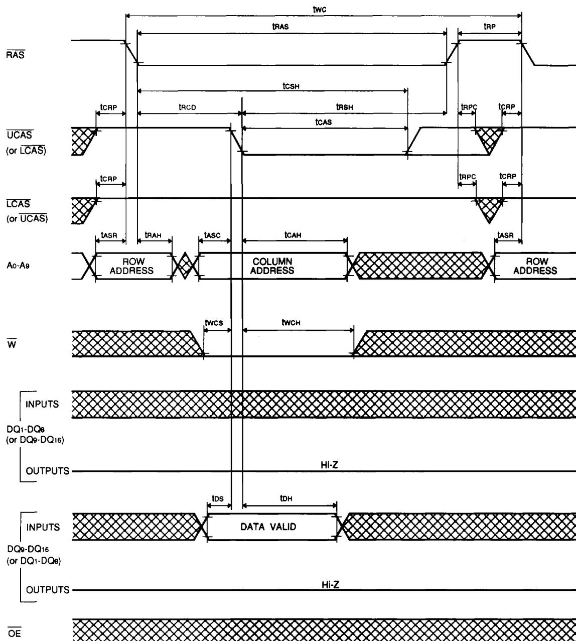
**Write Cycle ( Delayed write )**
