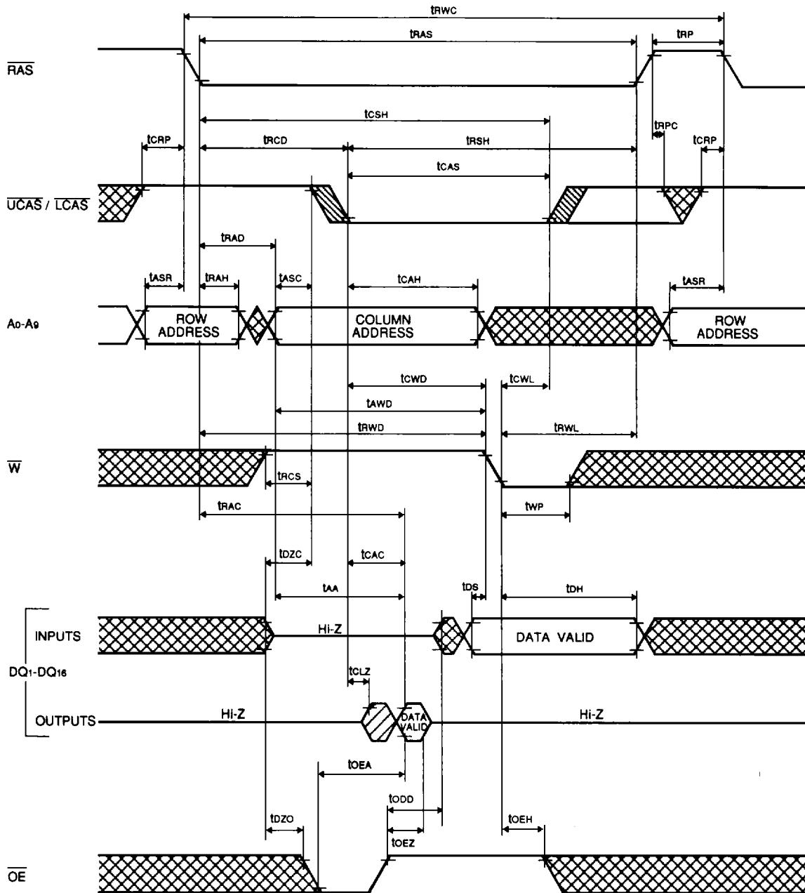
**Read-Upper/(Lower) Write, Read-Modify-Upper/(Lower) Write Cycle**
