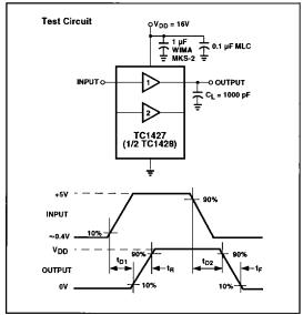
Figure 2. Non-Inverting Driver Switching Time
