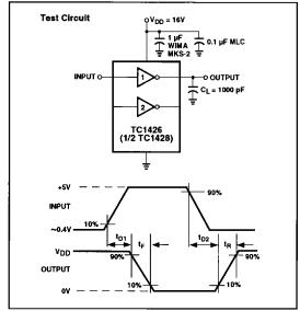
Figure 1. Inverting Driver Switching Time
