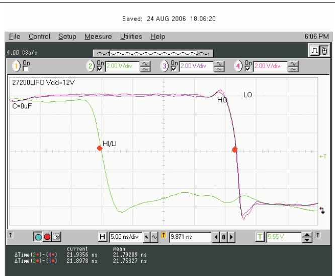
Figure 31. V_{LO} and V_{HO} Falling Edge Delay Matching
