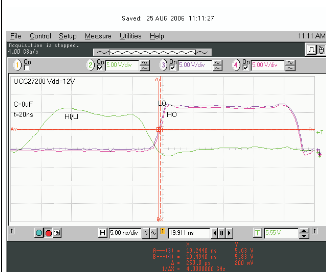
Figure 32. 20-ns Input Pulse Delay Matching
