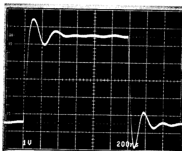
A_V = +10 , IN DEMO BOARD, R_L = 1k\Omega
