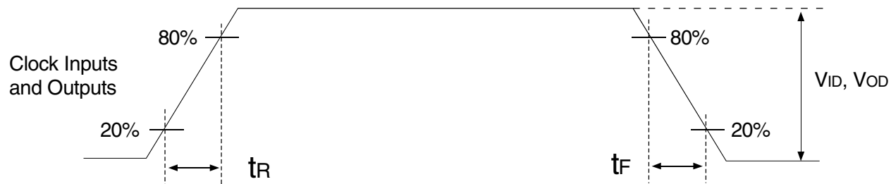
Figure 8. Input and Output Slew Rates
