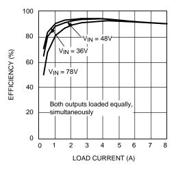
Figure 32. Total Board Efficiency
