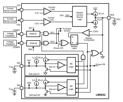
Figure 19. Current Limit Restart Circuit
