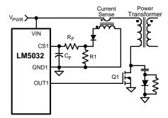
Figure 28. Current Sense Using a Current Sense Transformer
