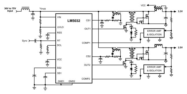
Figure 1. Dual Interleaved Regulators with Independent Outputs
