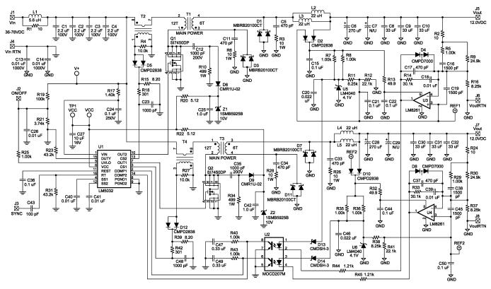
Figure 33. Dual Interleaved Regulator
