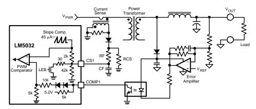
Figure 18. Typical Feedback Network
