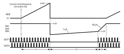
Figure 20. Current Limit Restart Timing
