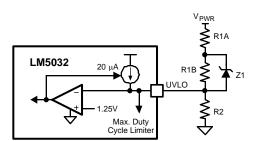
Figure 31. Altering the Slope of Duty Cycle vs. V<sub>PWR</sub>
