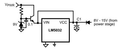
Figure 23. Start-up Regulator for V<sub>PWR</sub> >100V
