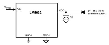
Figure 27. External Power to V<sub>CC</sub>
