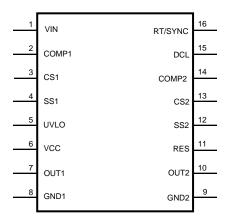
Figure 2. 16-Lead TSSOP (Top View) See Package Number PW0016A
