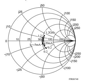
$\begin{array}{c} \text{S12e}: \text{V}_{\mbox{\scriptsize CE}} = 10 \text{V} \\ \text{f=} 200 \text{MHz step} \end{array}$
