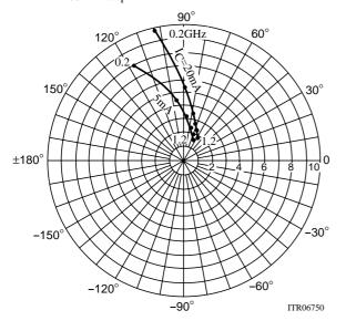
$\begin{array}{c} \text{S22e}: \text{V}_{\mbox{CE}} = 10 \text{V} \\ \text{f} = 200 \text{MHz step} \end{array}$
