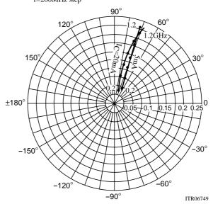
$\begin{array}{c} \text{S21e}: \text{V}_{CE} \text{=-} 10 \text{V} \\ \text{f=-} 200 \text{MHz step} \end{array}$
