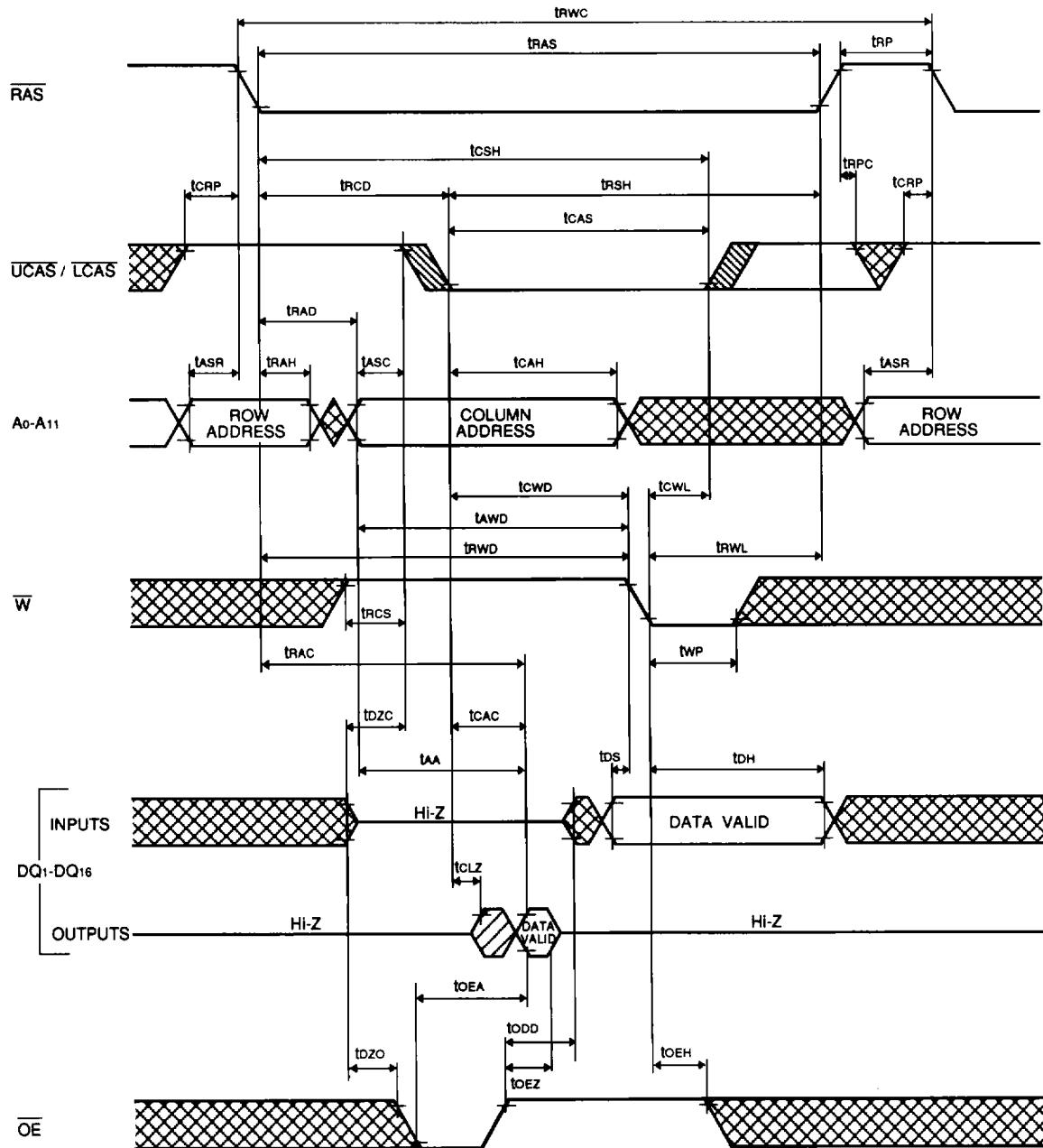
Read-Upper/(Lower) Write, Read-Modify-Upper/(Lower) Write Cycle
