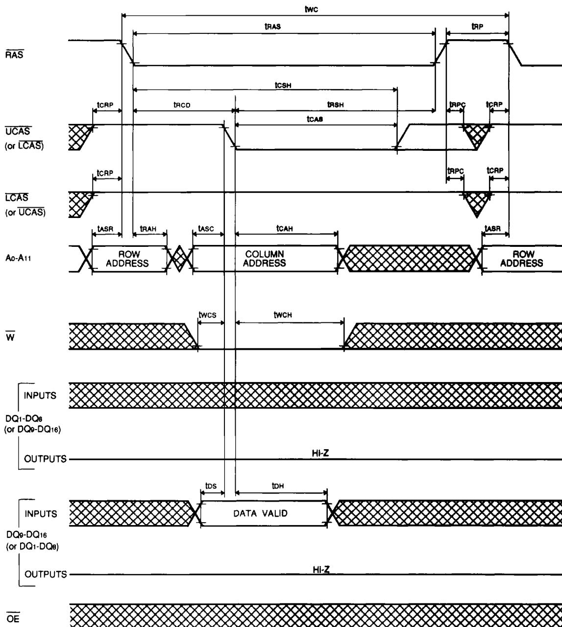
**Write Cycle ( Delayed write )**
