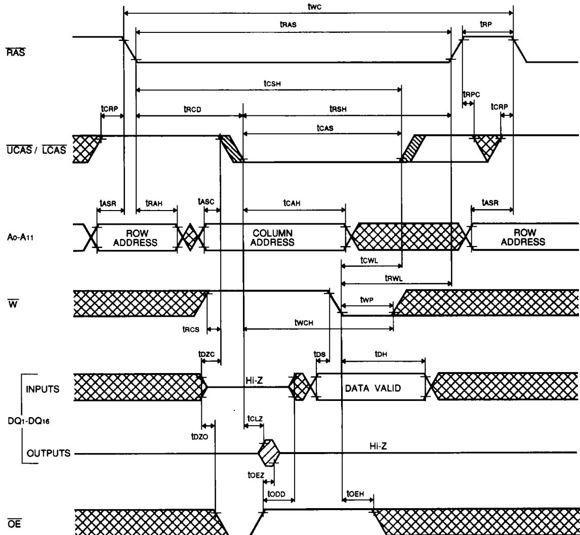
Upper/(Lower) Byte Write Cycle ( Delayed write )
