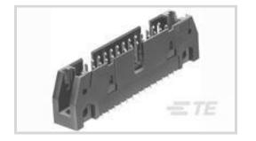
Connector System: Wire-to-Board Number of Positions: 34 Centerline (Pitch): 2.54 mm [.1 in ] PCB Mount Retention: With PCB Mount Retention Type: Screw Mount
