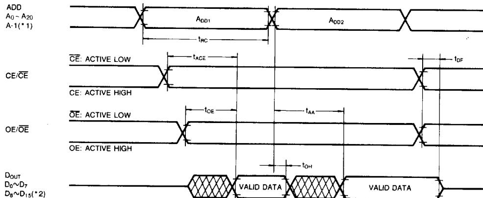
(\*1) Byte Mode only. A-1 is Least Significant Bit Address. (BHE=V<sub>IL</sub>)(\*2) Word Mode only. (BHE=V<sub>IH</sub>)
