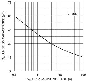
Fig. 5 Typical Junction Capacitance
