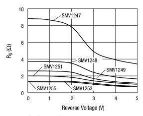
Series Resistance vs. Reverse Voltage @ 500 MHz
