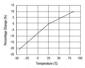
Relative Series Resistance Change vs. Temperature @ 500 MHz
