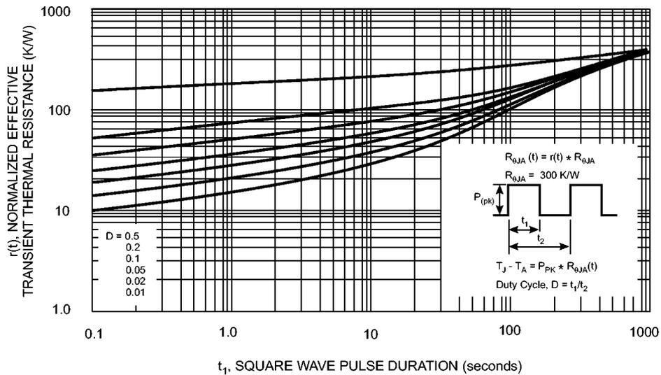
Fig. 4 Typical Normalized Transient Thermal Impedance Curves
