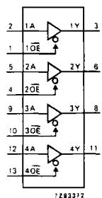
Fig. 4 Functional diagram.
