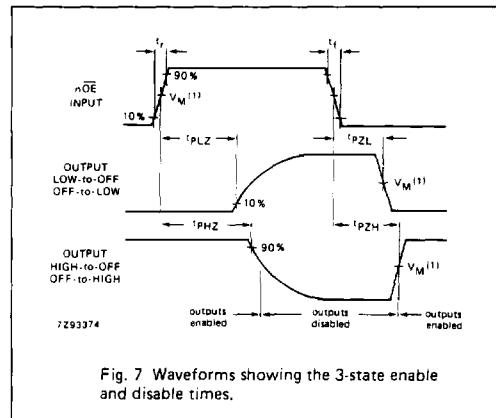
Fig. 7 Waveforms showing the 3-state enable and disable times.
