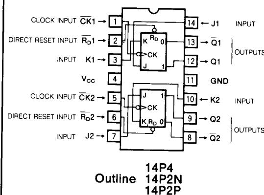
previous input at J and K appear at outputs Q and  $\bar{Q}$  in accordance with the function table given. When  $\bar{R}_D$  is low, Q and  $\bar{Q}$  will become low and high respectively, irrespective of other inputs. When used as a J-K flip flop,  $R_D$  should be maintained at high-level.
