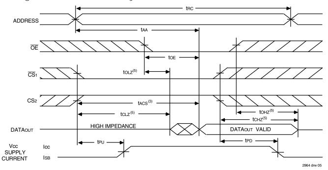
Timing Waveform of Read Cycle No. 2<sup>(1,2,4)</sup>
