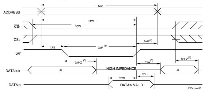
Timing Waveform of Write Cycle No. 2 (**CS**<sub>1</sub> AND CS<sub>2</sub> Controlled Timing)<sup>(1,4)</sup>
