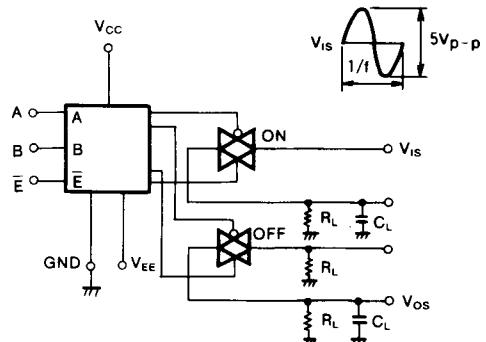
8. Low-level to high-level and high-level to low-level propagation time
