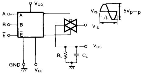
3. Low-level to high-level and high-level to low-level propagation time
