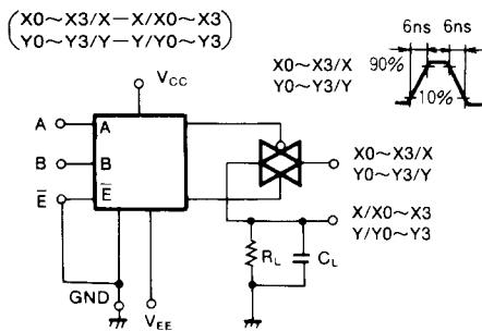
4. Low-level to high-level and high-level to low-level output propagation time, output enable, disable time
