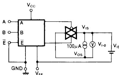
$$R_{ON} = \frac{V_{I-0}}{10^{-4}} (\Omega)$$
