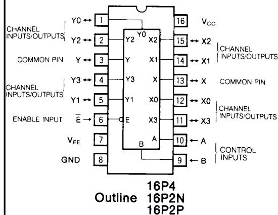
Analog signals of amplitude  $V_{CC} - V_{EE}$  greater than logic amplitude  $V_{CC} - \text{GND}$  at A and B can be switched.
