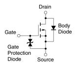
Remark The diode connected between the gate and source of the transistor serves as a protector against ESD.
