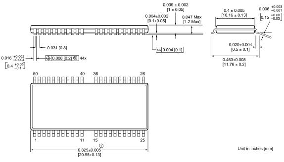
1 Does not include plastic or metal protrusion of 0.010 [0.25] max. per side
