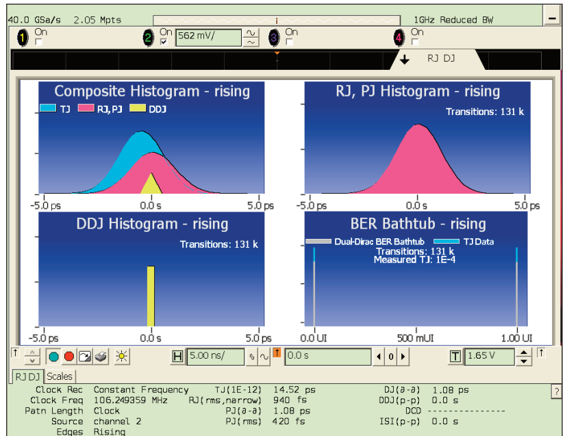
Figure 2: Jitter Analysis of a QT84L-106.25MHZ
